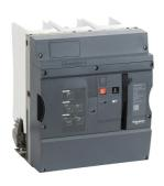
MV vacuum circuit breaker, EasyPact EXE, fixed, assembled, 12kV, 800A, 26.3kA 3s, 150mm, MCH 200VAC, MXF 24V
